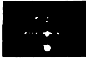
FIGURE 3 (a) Unshuttered growth. \approx \langle 110 \rangle SrTiO 3 azimuth. Composition Dy 0.18 Ba 0.33 Cu 0.49 O 7-x .
